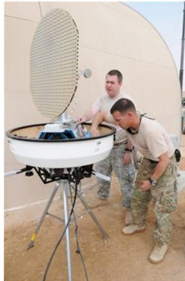
SOUTHWEST ASIA - U.S. Air Force Staff Sgt. Samuel Trammel and Tech. Sgt. Matthew Brown, U.S. Air Forces Central Weather Systems Support Cadre members, inspect a portable Doppler radar prior to installing it at the 380th Air Expeditionary Wing Sept. 12, 2012. Doppler radar will allow the 380th Expeditionary Operations Support Squadron Weather flight to interrogate a storm and gather real-time storm data. (U.S. Air Force photo/Tech. Sgt. Amanda Savannah)
